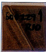
(above) Many slates bleach during acid tests — Wang Wei Green
