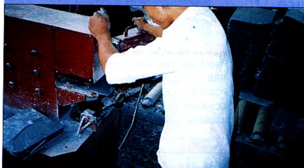
Cutting Chinese slate (above) and (below) Pre-holing of slate using drills. Note the curvature to some slates in the pile on the left.
