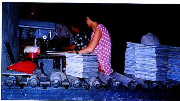
Cutting Chinese slate (above) and (below) Pre-holing of slate using drills. Note the curvature to some slates in the pile on the left.
